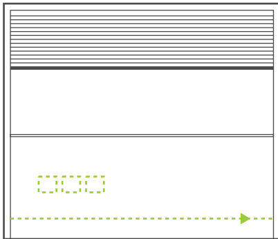
Cabling and socket cut outs at floor level
